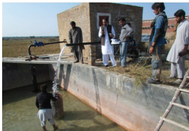
Technicians and farmers watch as an alternating-current solar-powered pump meant to be used with a high-efficiency sprinkler irrigation system is tested at a farm in Talagang, Pakistan, in December 2015. (Photo: HI-AWARE project team/Pakistan Agricultural Research Council)
